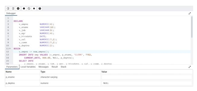
The debugger may be used to debug PL/pgSQL functions in PostgreSQL, as well as EDB-SPL functions, stored procedures and packages in EDB Postgres Advanced Server. The Debugger is available as an extension for your PostgreSQL installation, and is distributed as part of Advanced Server. You must have superuser privileges to use the debugger.
